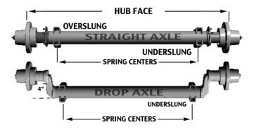
Alternatively - the flange face to flange face measurement can be provided which is measured from the outside of one brake flange to the outside of the opposite one (Where the brakes bolt on) as you see below.
